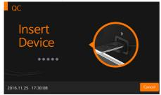
When the test device is inserted into the analyzer, the analyzer will automatically check whether the device is unused or not. Also, the analyzer will read the barcode data and confirm the test device is valid before starting the test.
