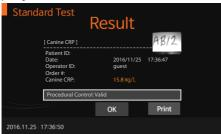
When the 'OK' button is pressed, 'Eject Device' will be displayed. The test device can then be removed from the analyzer.
