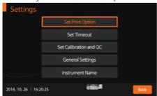
To set the number of printed sheets as 1, 2 or auto-printing mode (ON/OFF) enter the 'Set Print Option' menu. Auto-printing means the built-in printer will automatically print all test results at the end of each test.
