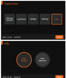
When 'View Version' is selected, the version information for the software and firmware will be displayed. Press'OK' to confirm.
