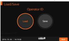
When the operator's ID is loaded, the screen will promptly show a message indicating that the operator's ID has loaded successfully. Press'OK' to confirm.
