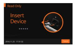
4. When inserting the test device into the analyzer, the analyzer will automatically check whether the test device has been used previously or not. The analyzer also reads the barcode data and confirms the test device is valid before starting the test.
