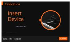
When the device is inserted into the analyzer, the analyzer will automatically check whether CAL-1 is unused or not. Additionally, the analyzer will read the barcode data and confirm the device is valid before starting the calibration set test.
