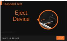
10. When the test device is ejected, the analyzer will move to another test log-in menu for the next test. Press'Cancel' at any time to stop the test progress.
