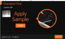
The analyzer automatically recognizes the test device. The time required for analysis depends on type of test device.
