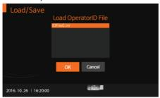
In addition, the operator can save the operator's ID by pressing 'Save'. When operator's ID is saved, press 'OK' to confirm.
